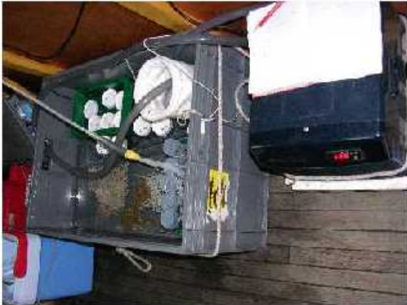
Onboard incubations to determine calcification rates using ambient seawater
