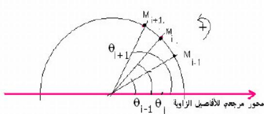
$$\omega_i = \frac{\vartheta_{i+1} - \vartheta_{i-1}}{t_{i+1} - t_{i-1}}$$
