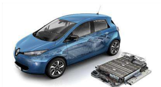
Zoé 400 V, 41 kWh, 12 modules, 192 cellules, 290 kg
