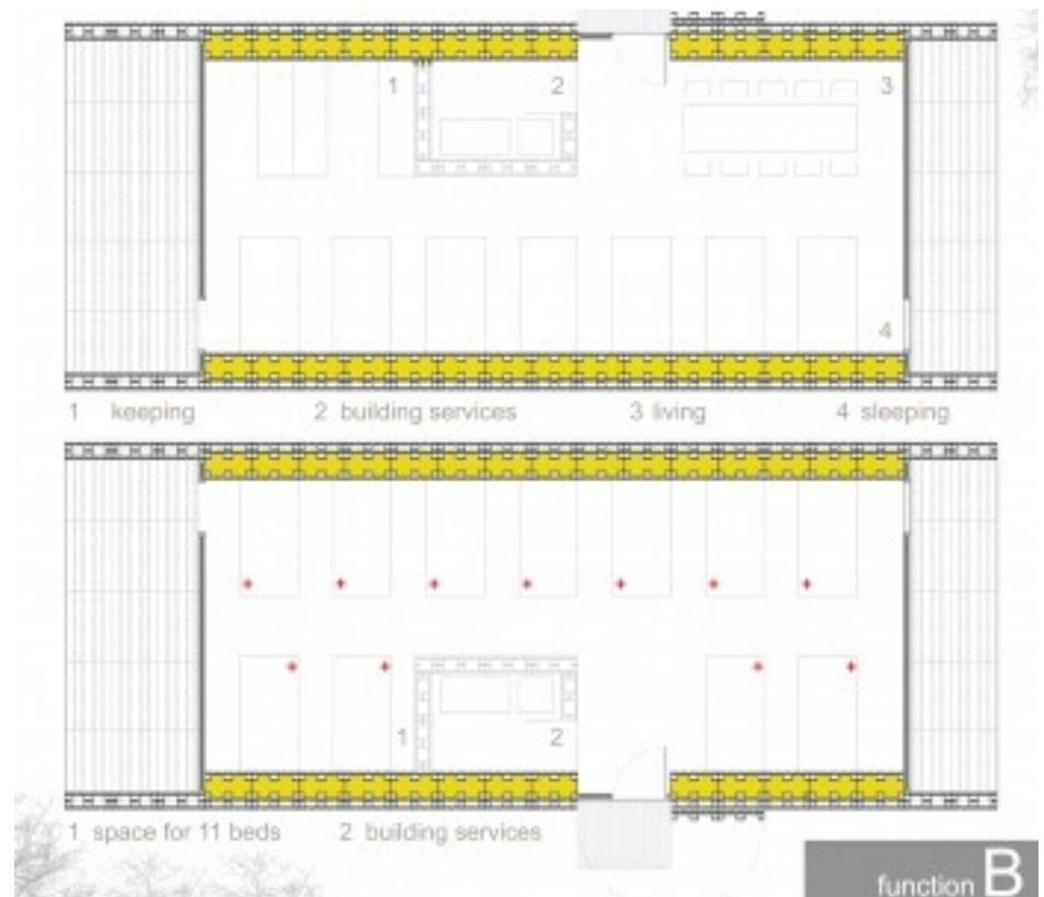
Layout plan (ground floor) 1:200
