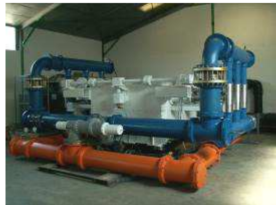
Fig 16 – 5 MLD Boxer pump with Integrated Isobaric cylinders.
