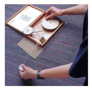
You spin off the point of a charkha's spindle. The device is like a turbocharged handspindle, and is well suited for spinning fine, high-twist yarns. Underneath this one-box charkha is the textured shelf liner Marilyn uses to keep the charkha from sliding around when she spins—a good tip for any small wheel.
